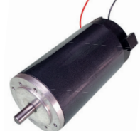
AT 1503 Motor imã permanente 260Vcc 1400W 3200 RPM 71B14 Ø 102,0 CW/CCW
